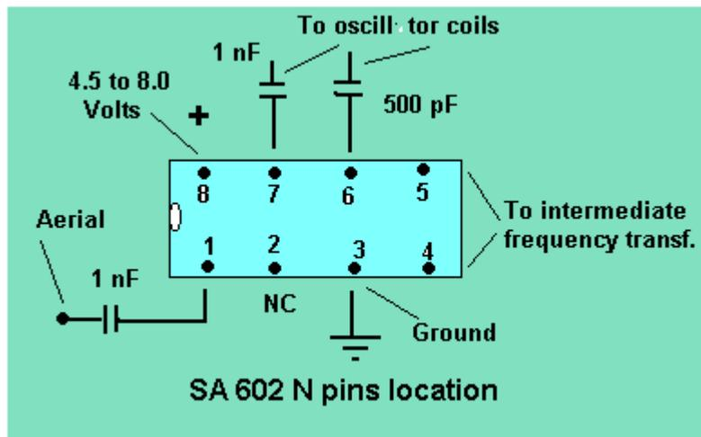
Though the SA602N can work from 4 to 8 volts, the most appropriate voltage for this project is 6 volts. Pin #2 is not connected and the negative pole of the 6 volt battery is plugged to ground.
