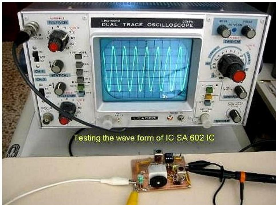
Also, between Pin #4 and Pin #5, you can obtain the wave form in the picture to the right.
