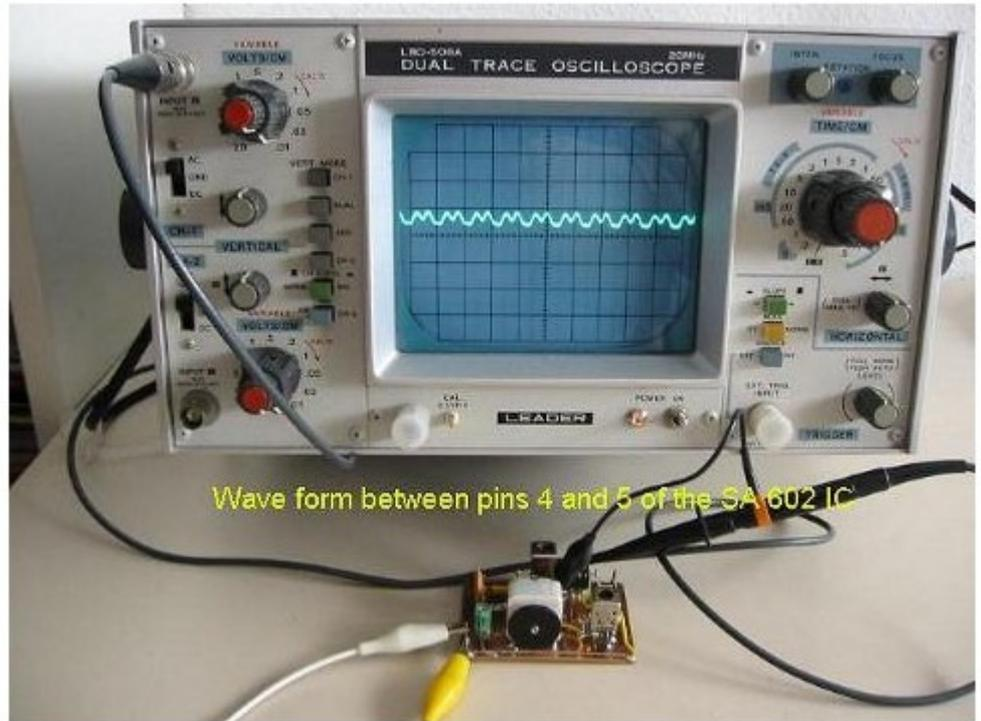
***Finally, the SA602N IC opens a wide field of experimentation due to its' capacity to oscillate up to 200MHz. You can build with it short wave, FM and higher frequency receivers. This circuit allows also the building of direct convesion receivers.***
